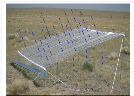
**Fig. 2.** Example of a simple, passive precipitation reduction shelter that removes a fixed proportion of each rain event (blue dotted lines represent rainfall) from reaching experimental plots. This basic design, modified in scale and placement (i.e., below the canopy in forests), has been used successfully in a wide range of ecosystems.
